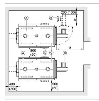
To enable convenient installation and maintenance, observe the stated clearance dimensions; maintain the minimum clearances where space is tight (dimensions in brackets). In the delivered condition, the boiler door opens to the right. You can reposition the hinge pins so that the door opens to the left.
