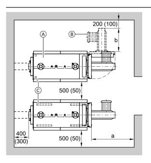
To enable convenient installation and maintenance, observe the stated clearance dimensions; maintain the minimum clearances where space is tight (dimensions in brackets). In the delivered condition, the boiler door opens to the left. You can reposition the hinge bolts so that the door can open to the right.
